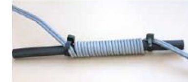
Speaker wire wound around ferrite rod
