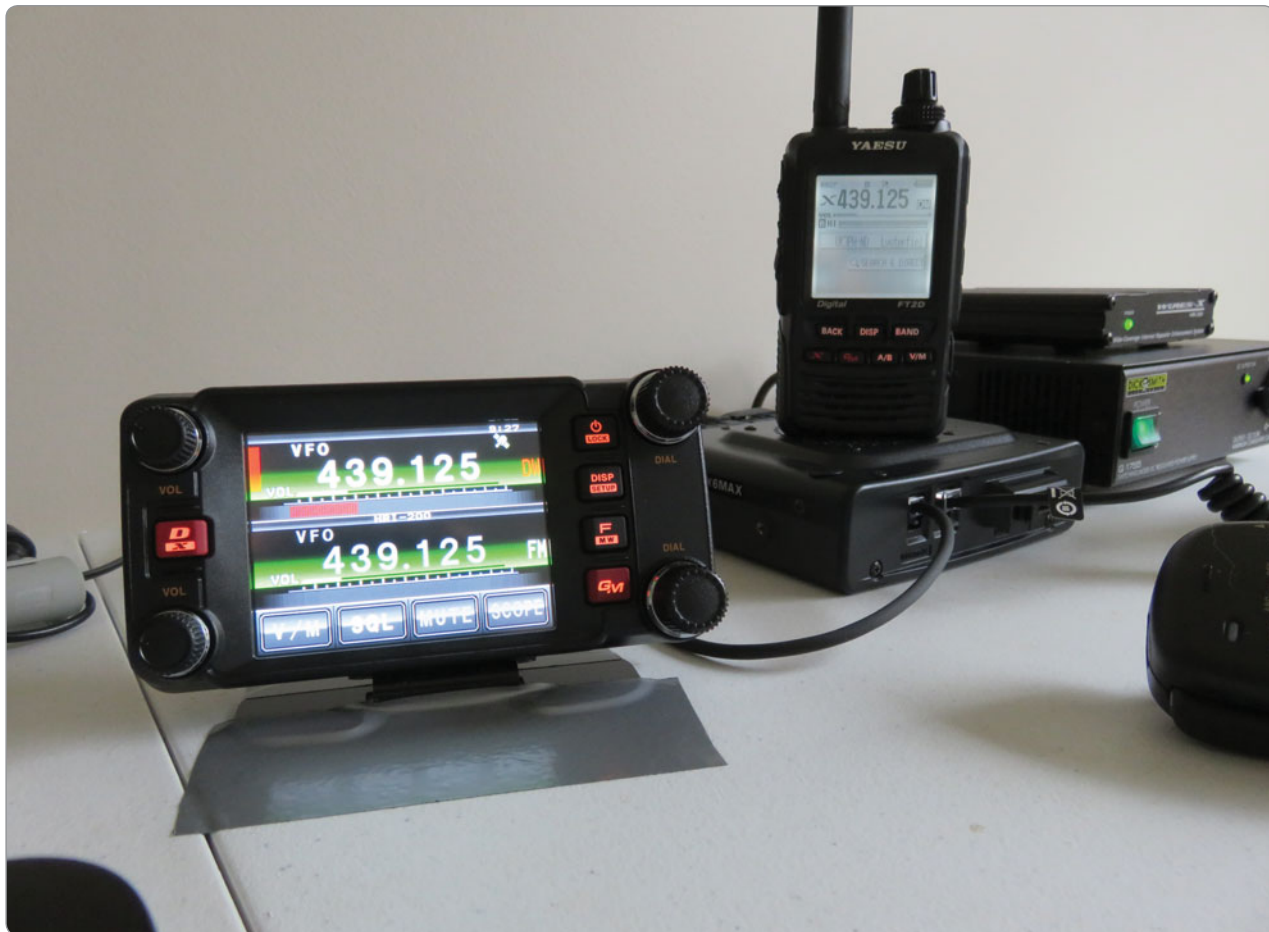
Photo 3: The transceiver and associated equipment set up to operate as a WIRES-X radio node.
