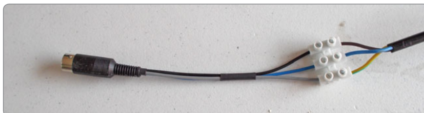
Photo 6: Terminal block to 5 pin DIN connector.
